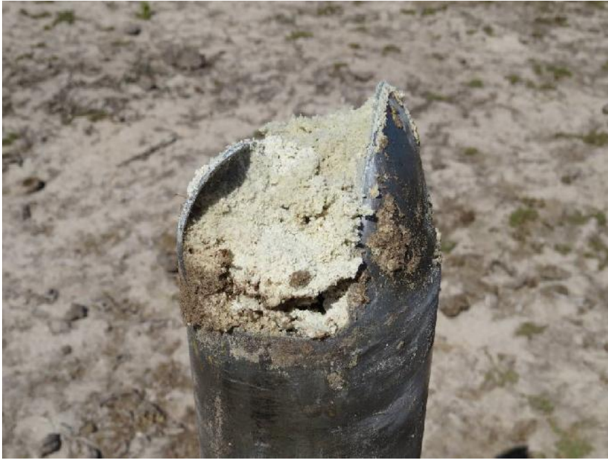
Photograph 1: Soft Carbonate Horizon
