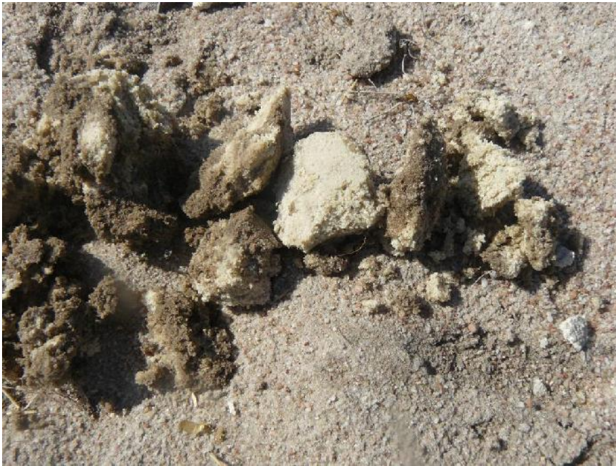
Photograph 2: Saturated soft carbonate horizon
